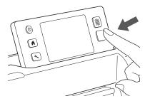
When cutting is finished, the message "Finished cutting." appears on the display. Touch the "OK" key to return to the draw/cut selection screen.
